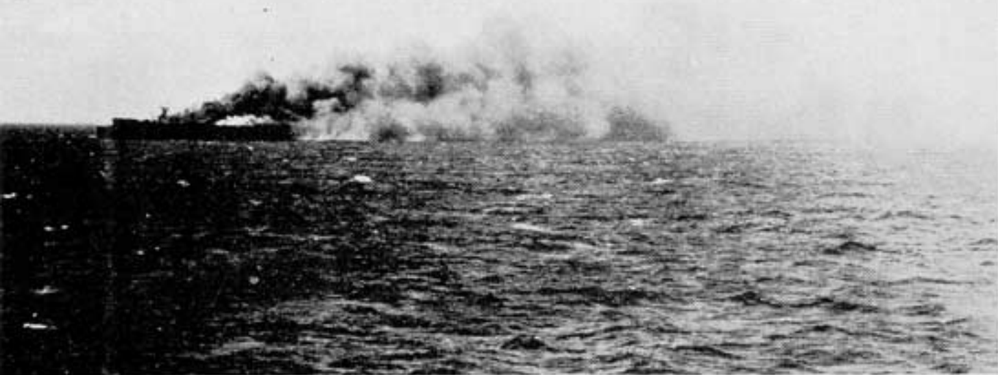
3. PRINCETON at about 0953. Fire raging aft. Ship has turned to put wind 45 degrees on port bow. Smoke appears to be blowing clear of the ventilation supply intakes on the port side.
