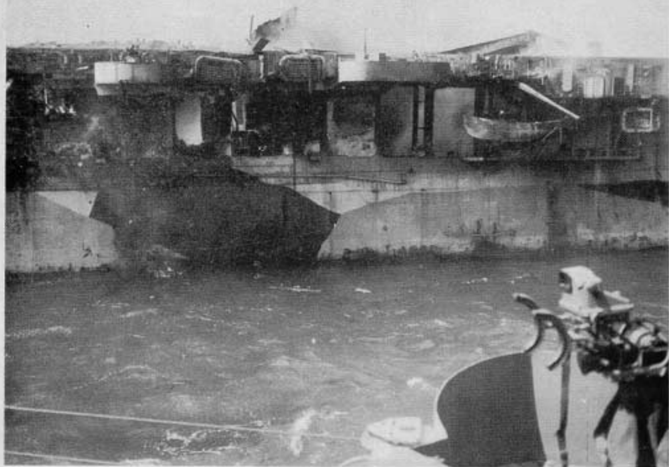
11. View of after port side of PRINCETON. Note hangar roller curtains demolished, panel between frames 110 and 113 blown out and hole in panel between frames 115 and 118.
